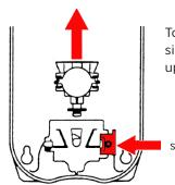
To release valve, push in side catch and lift valve upwards.
