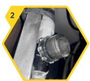
Remove cap from injection fitting
