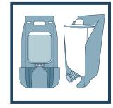
Fit a new cartridge or fill the reservoir with hand wash, replace top of reservoir.
