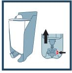
Bulk fill dispenser: Press the release fitting to remove the connected reservoir and valve.
