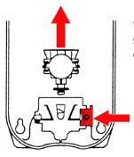
To release valve, push in side catch and lift valve upwards
